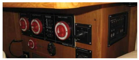
Battery, Gen, Windless and Elec Winch Switches
