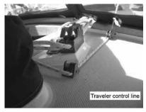
port and starboard orientation. I had to rethread the control line on the traveler so it would come over the top rather than through it. Photos 8 and 9 show the new arrangement.
