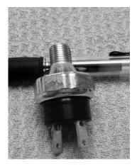
the electric fuel pump. If the contacts open with the engine running your low oil pressure alarm will activate and there will be no DC power to the electric fuel pump. The engine may run for a while with the pump not running, but sooner or later the engine will sputter, rpm will fall/rise and it may shut down or just loose power."
