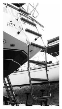
Design for new bi-folding ladder that would extend 3 rungs below the water-line.
