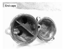
water injection point. The metal was not only cracked but was spongy. It was not repairable. There have been a few changes to the design of the mixer over the life of the C42. The version that Catalina had in their spare parts stock did not exactly match the leaking part on *Mi Vida*. Therefore I had a replacement fabricated at Metal Magic, a local SF Bay area shop. The Catalina spare part could have been made to work, but it would have required a relocation of the muffler.
