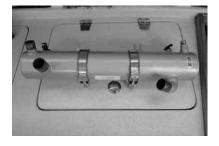
out with a new bracket system. The new system is a steel band that wraps around the HE and bolts in as before. After reinstalling the HE with the new brackets, I won't go into the level of difficulty; the HE sits back further cramping the exhaust hose. The same issue of vibration still works steel against bronze and within 2 years it was leaking again.
