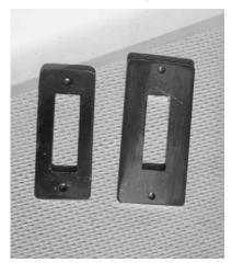
After I finished the project and stood there admiring my work I was hit with a "Homer Simpson" moment! Dooooh! I should have done what Don Casey suggests, over drill the holes, fill them with epoxy and then drill new holes for the cover plate screws into the epoxy. This will eliminate any water getting into the
