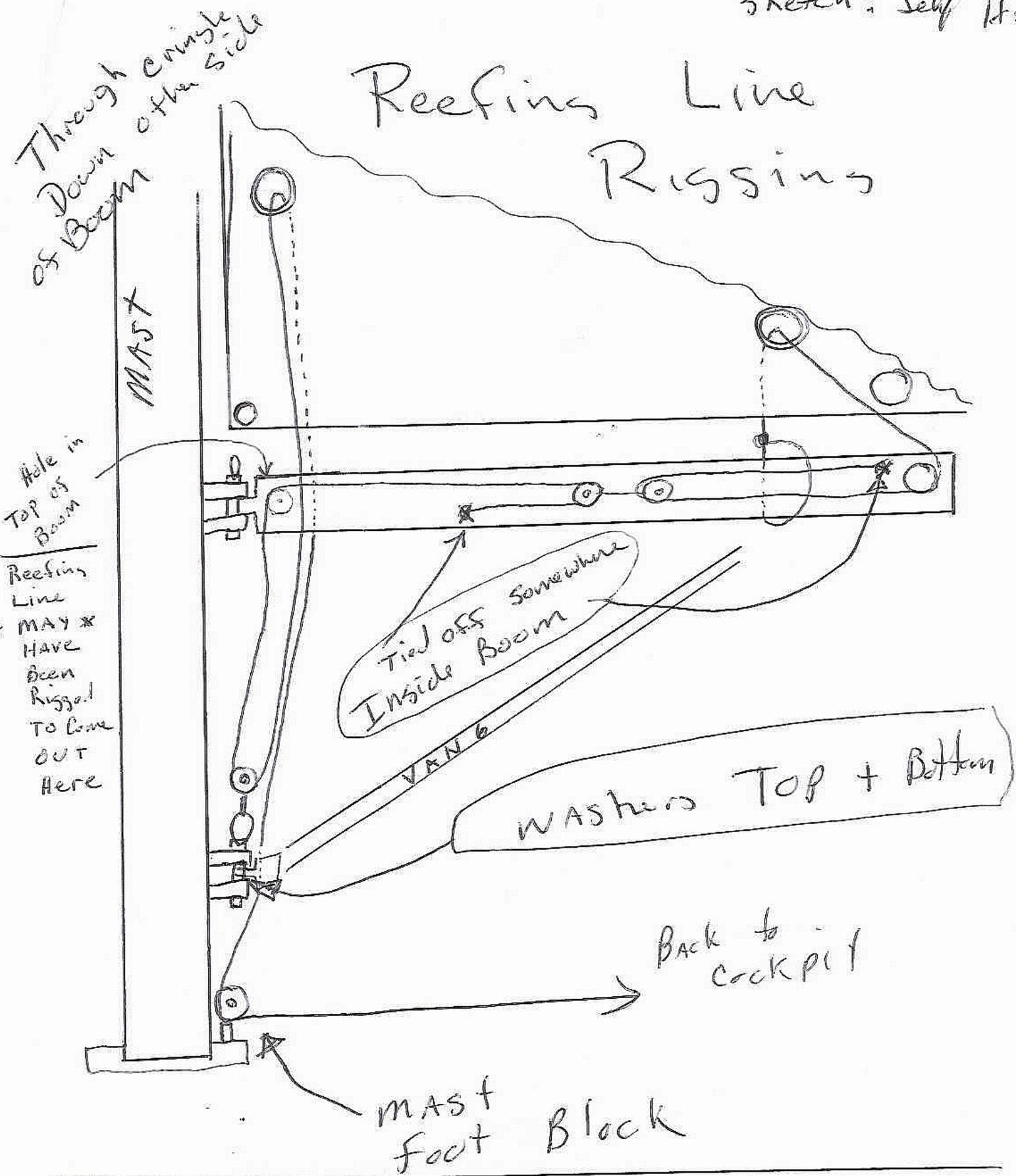
Notes: This Arrangement is used when there ~~are~~ only 1 Reefing Line exiting each end of the Boom, with other ~~lines~~ Ends tied inside the Boom
